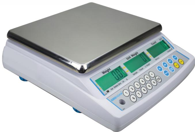
The CBC bench counting scale offers intelligent functions that are practical for any counting application. The intuitive software is user-friendly and keeps track of the count, automatically optimising the unit weight for greater accuracy. Designed to be tough, the CBC features ABS housing, stainless steel platform, non-slip feet and load cell protection. RS-232 interface allows easy communication with computers and printers.
